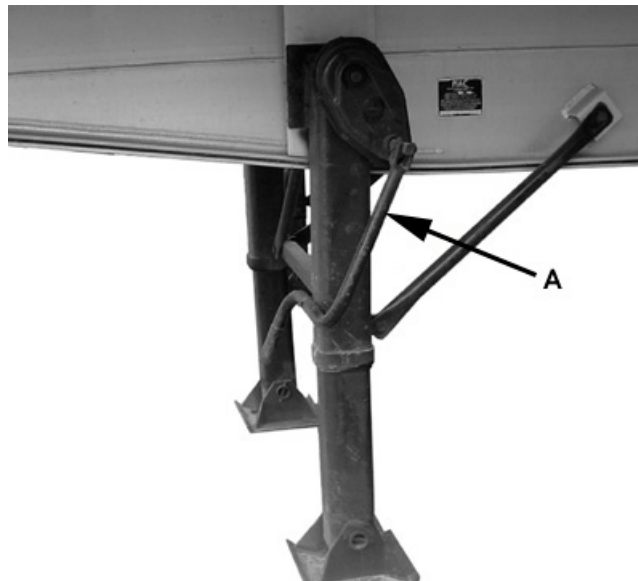
Figure 3-7 Two Speed Landing Gear
