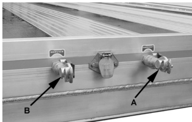
Figure 6-2 Disconnect Hoses And Electrical Connector
